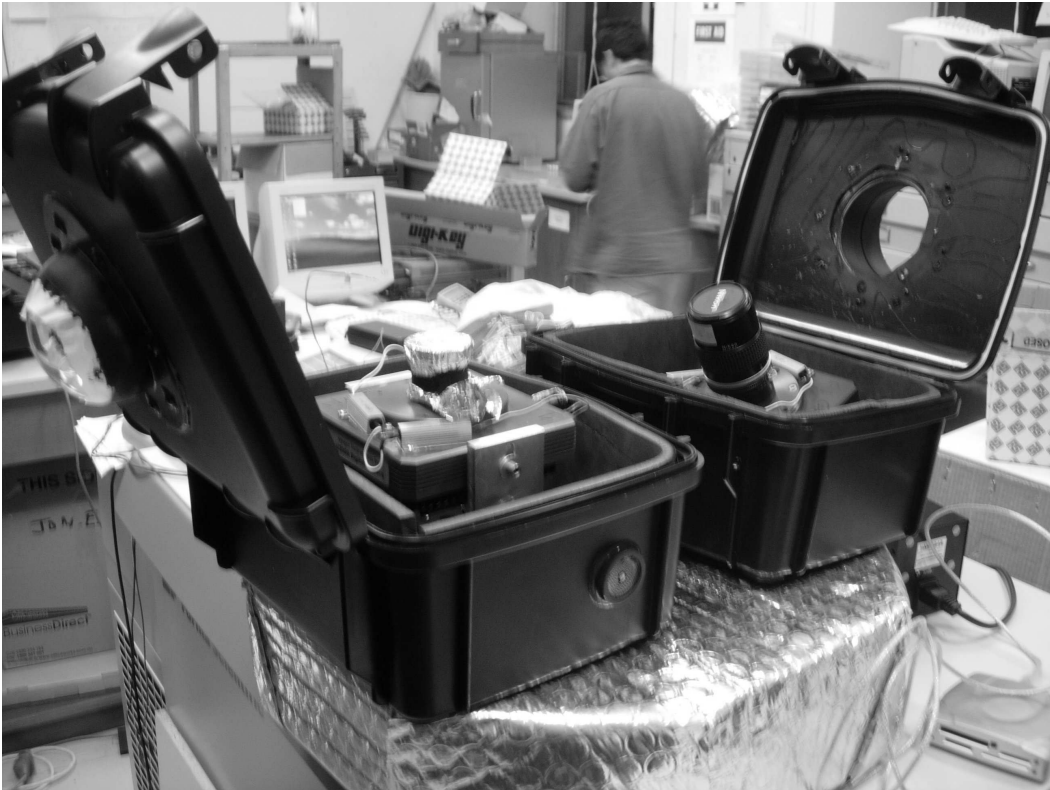
Figure 2.2: The two cameras in their enclosures in the lab at UNSW. The all sky camera is on the left and the SBC is on the right.
