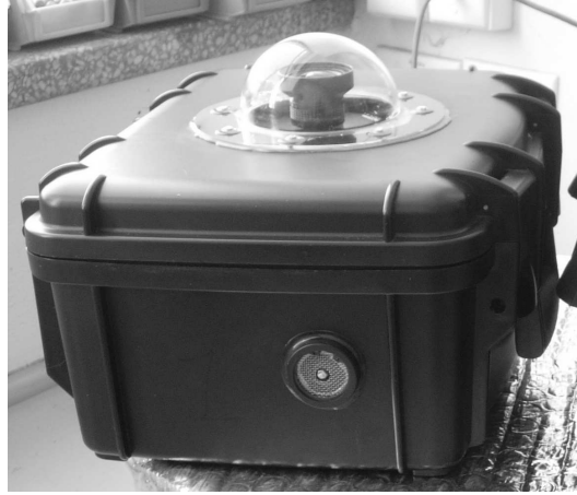
Figure 2.4: The all sky camera in its enclosure.
